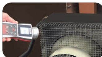
Stroboscope off: rotations not visible
