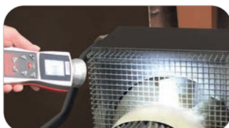
Stroboscope on: rotations visible
