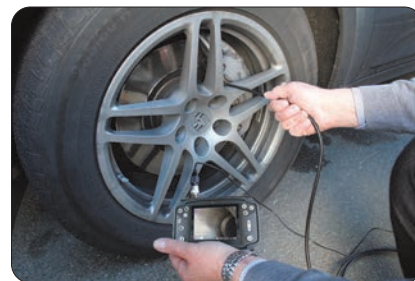
Example: brake discs control
